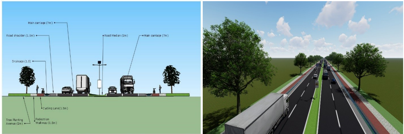
Plate 4-12: Sample cross section of 30 Metre Road
